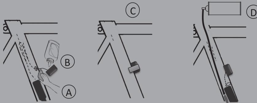
A: Follow the instructions on the adhesive carefully in relation to cleaning, and mixing and curing, if necessary. B: Apply the appropriate layer of adhesive on the antenna. C: The antenna is placed over the hole and the cable is hidden in the frame below the antenna. Hold the antenna lightly with tape until the adhesive has hardened. D: Place the cable neatly into the seat tube and lightly foam the tracker (avoid foaming the cable).
