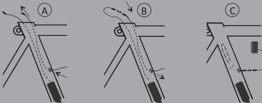
Possible ways to pull the antenna cable out: A: Pull a cable puller through the frame and screw onto the cable. B: Pull the antenna cable carefully through the hole and remove the cable puller. C: Connect the tracker and antenna by screwing the cables together.
